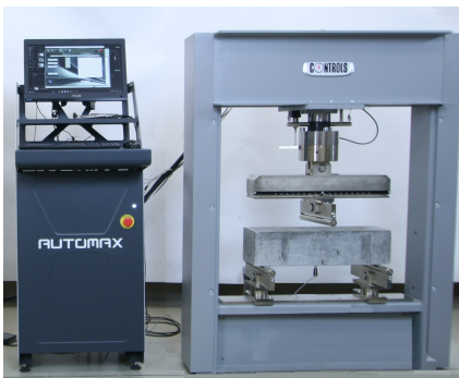
50-C20M82 AUTOMAX MULTITEST controlling a 350kN flexure frame for FRC testing
