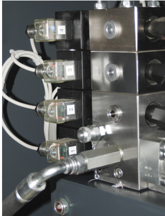
50-C10D/3F AND 50-C20E/4F hydraulic valves for connection and control of four frames
