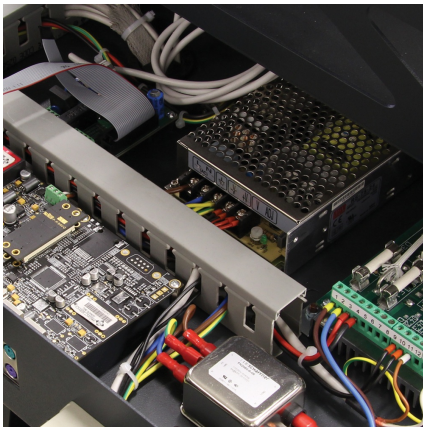
Detail of electronic boards housed in the removable drawer of Automax MULTITEST console
